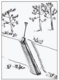
Illustration 4. Water bar installation Proper installation of water bar.
